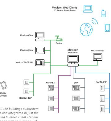
The flexible architecture of Movicon ™ BA allows all the buildings subsystem including networks and various devices to be concentrated and integrated in just the one all-inclusive supervisor. Information can be distributed to other client stations such as PC, touch screen panels, mobile devices as well as over the web.
