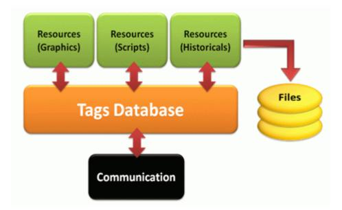
This block diagram outlines the Movicon platform architecture and structure.
